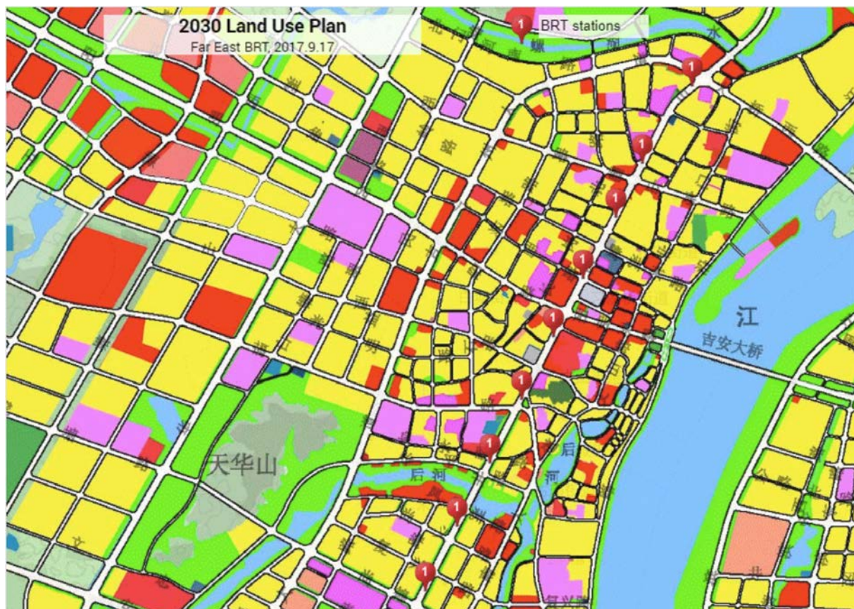
Figure 24: Example of land and function mix by block and within block in Ji'an, Jiangxi province, People's Republic of China (zoning map 2016–2030). 40
