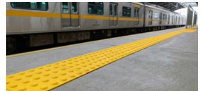
Figure 99: Tactile warning tiles on platform edges 127
