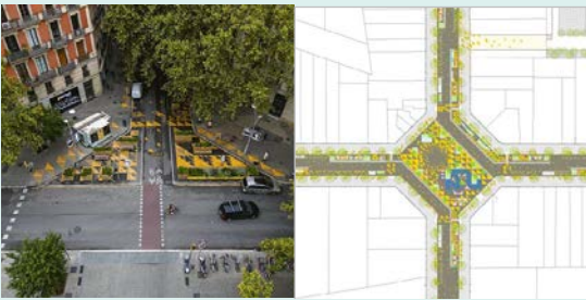
Figure 40: Modal filter and restricted turns on: Carrer del Comte Borrell. Part of Sant Antoni Superblock in Barcelona 56
