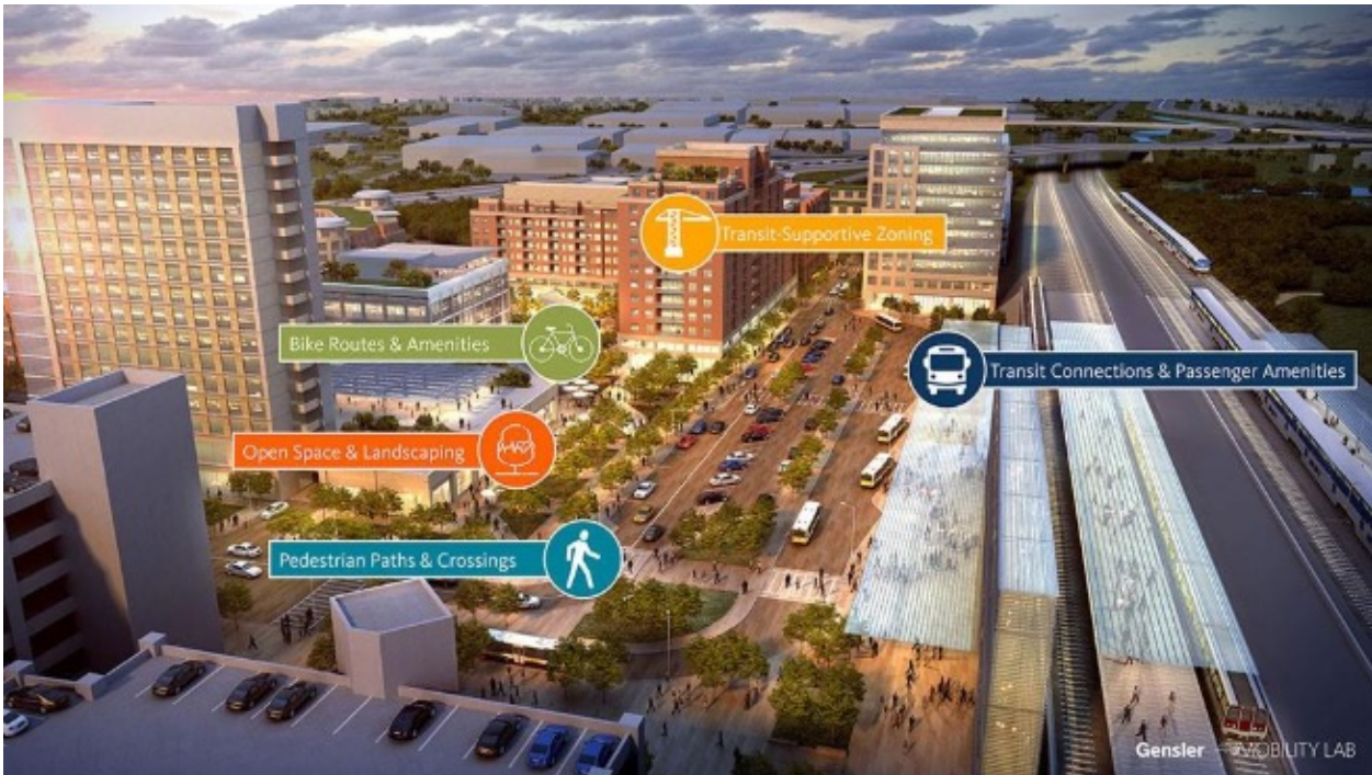
Figure 49: Illustration of station-centred development; public transport, bicycle and pedestrian priority, compact development and mixed-use integration 71
