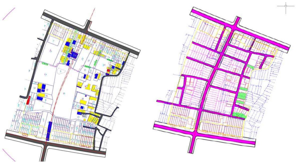
Figure 28: Land readjustment in the normal area (illustration of land readjustment in Tra Vinh) 46
