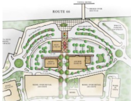
Figure 78: Transit-oriented development urban structure with parking and amenities for vehicles of the first-mile/last-mile 100
