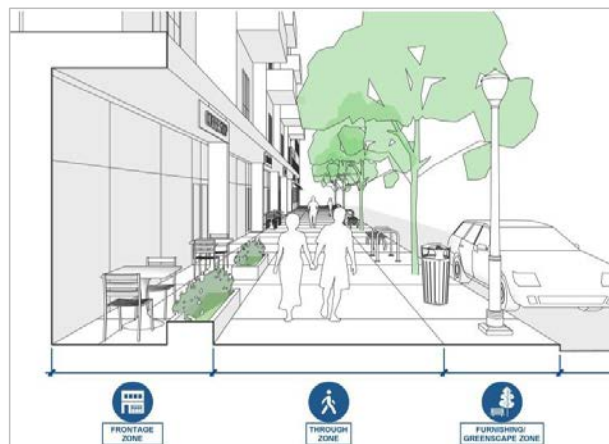
Figure 38: Example of providing an unobstructed pedestrian path alongside trees, street furniture and active frontage 54
